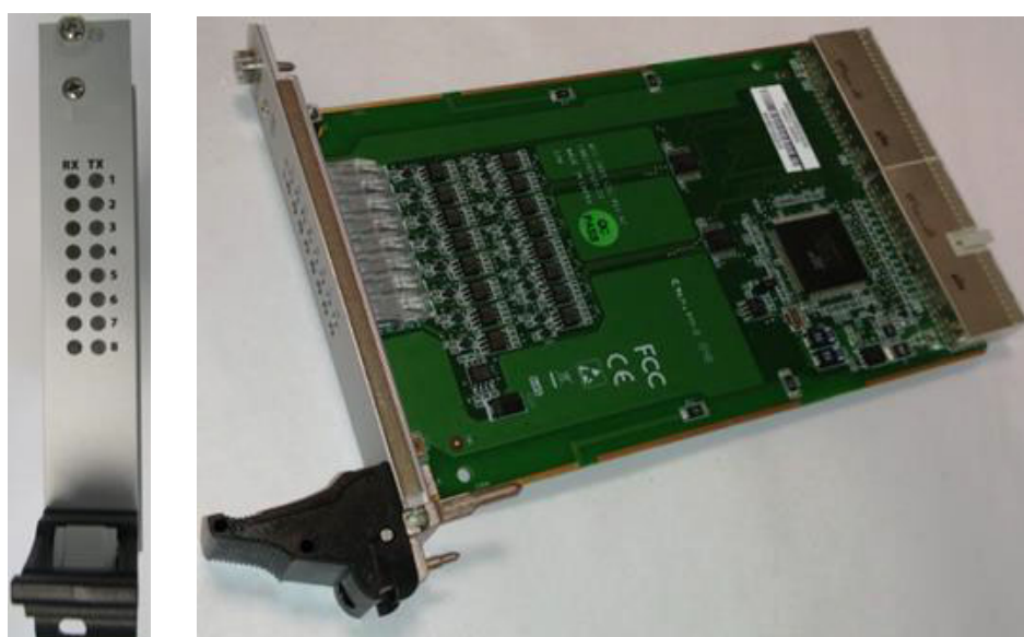
Figure 2.8 MIC-3955 FIO, for 8 port DB37 pin RIO
