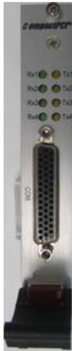
Figure 2.9 Rear IO MIC-3527A1 for MIC-3955 4-port DB44 female connector via backplane
