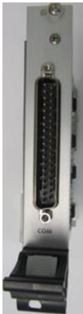
Figure 2.10 Rear IO MIC-3527A2 for MIC-3955 8 port DB37 male connector via backplane
