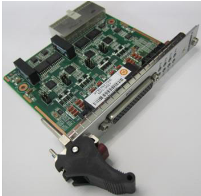
Figure 2.9 Rear IO MIC-3527A1 for MIC-3955 4-port DB44 female connector via backplane
